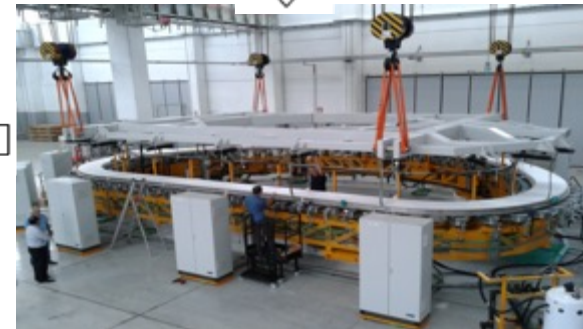
DP Loading into Vacuum Impregnation Mold (radiation- hard cyanate ester resin)
