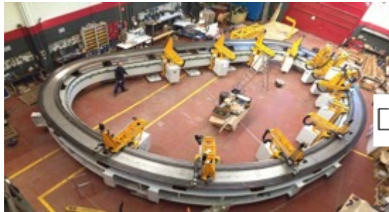
DP Turn Insulation inside Radial Plate
