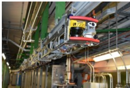
Train Inspection Monorail (CERN made)
