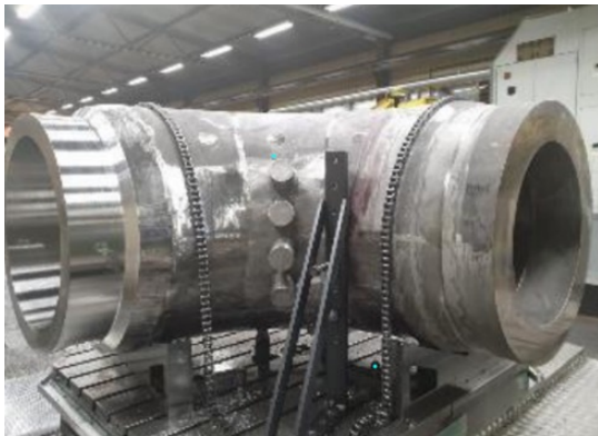
Framatome, Primary circuit elbow manufactured via HIP [1]
