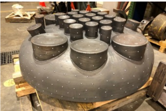
EPRI, SMR Upper Head blank produced via HIP [2]
