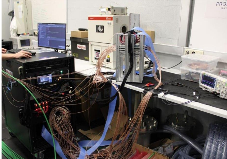
Test tower containing test samples being characterized at different T and V levels before irradiation experiment.
