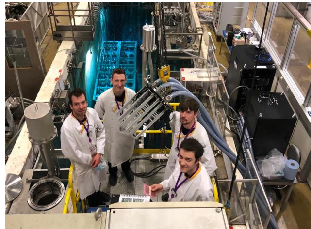
Test tower containing test samples being characterized at different T and V levels before irradiation experiment.
