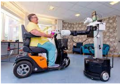
Robust and safe remote-control system for elderly people assistance (Heemskerk Innovative Technology)
