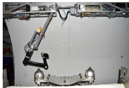
TIM robotic arm equipped with HD camera
