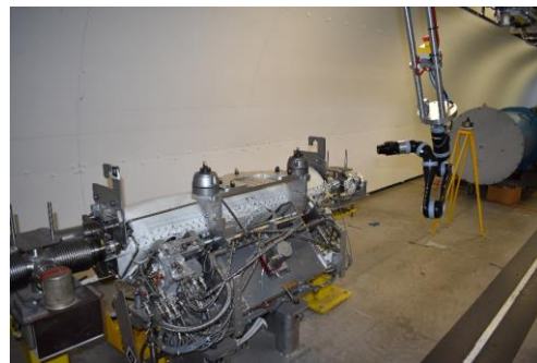
TIM robotic arm for survey on LHC collimator
