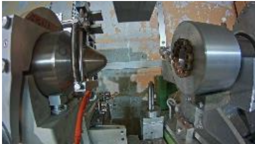
Temperature sensor installation on AD target
