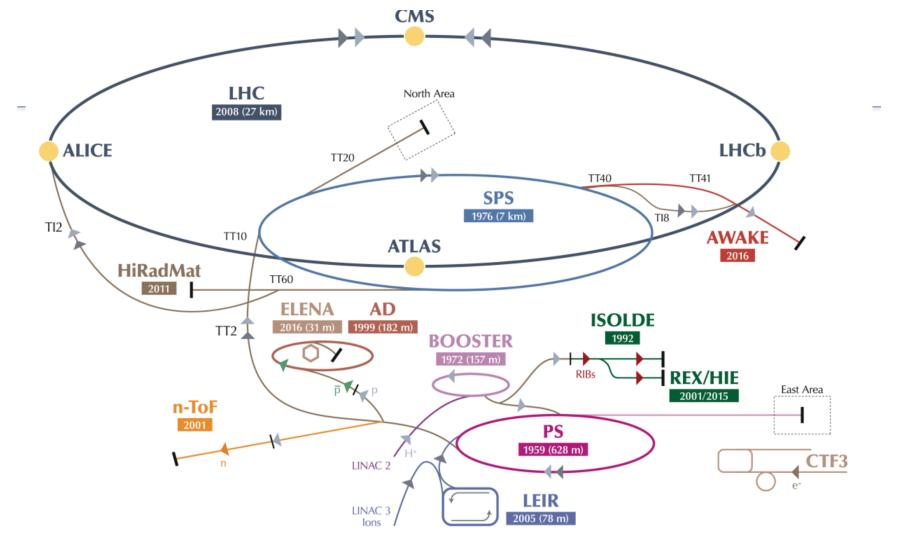
~250 devices scattered from the Linac source stopper (45 keV) to the LHC main dump (7 TeV)
