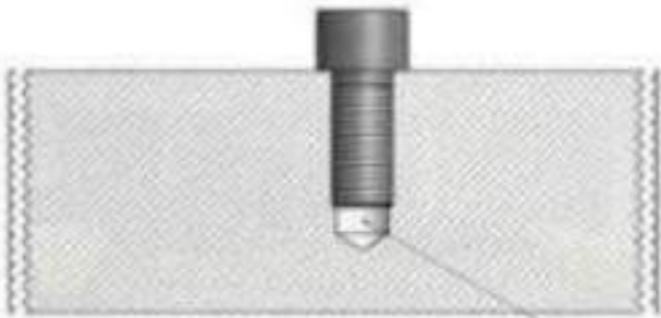
Trapped volume tortorous leak path trough threads
