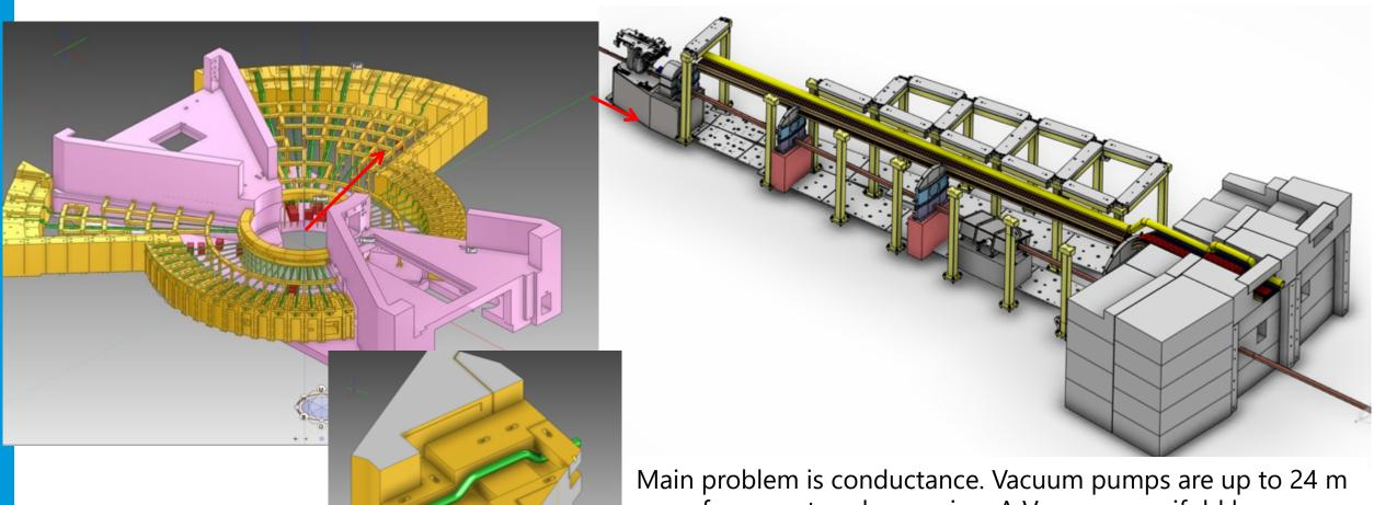
Main problem is conductance. Vacuum pumps are up to 24 m away from neutron beam pipe. A Vacuum manifold has limited space to go through the bunker wall. Vacuum specification equivalent to UHV, same as particle accelerators including material limitations on the chambers sealing due high activation by neutrons.
