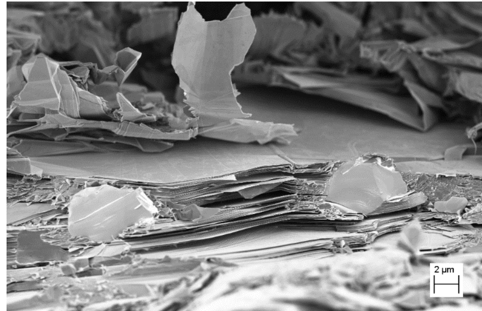
Perpendicular fracture surface
