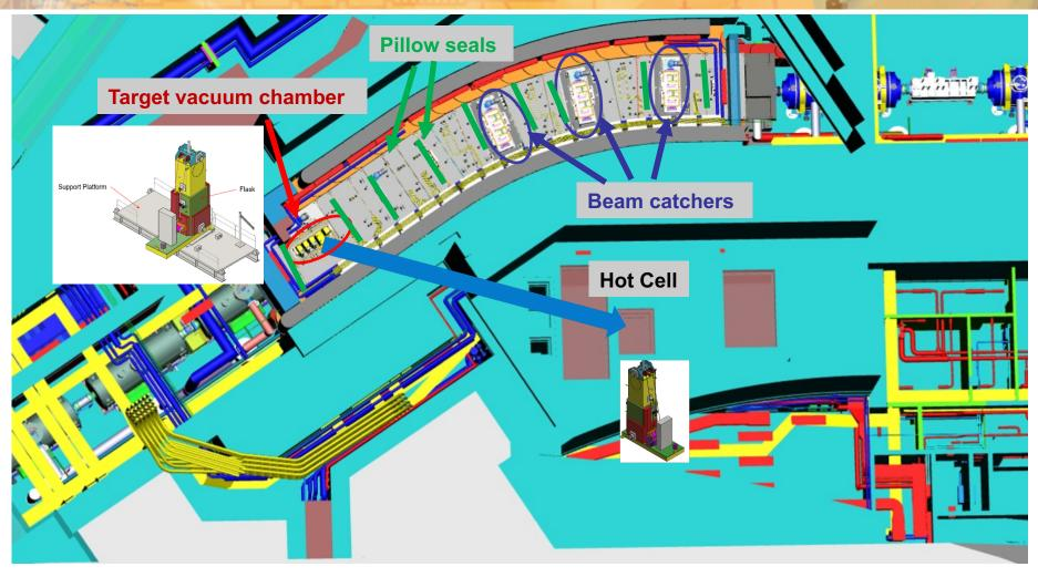
The components will be moved in the shielding flask from the beam line to the hot cell and be indserted through the double lid slider of roof
