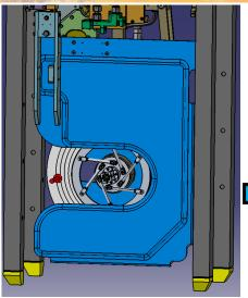
**Step 1:** cooling plate removal
