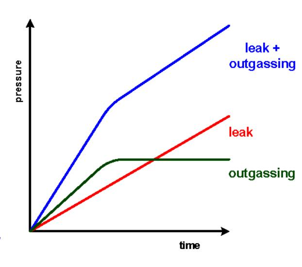
The leak rate is defined as the pV throughput of a gas through a leak. It is a function of the type of gas, pressure difference, and temperature. In a system of volume V the leak rate  $Q_i$  is given by
