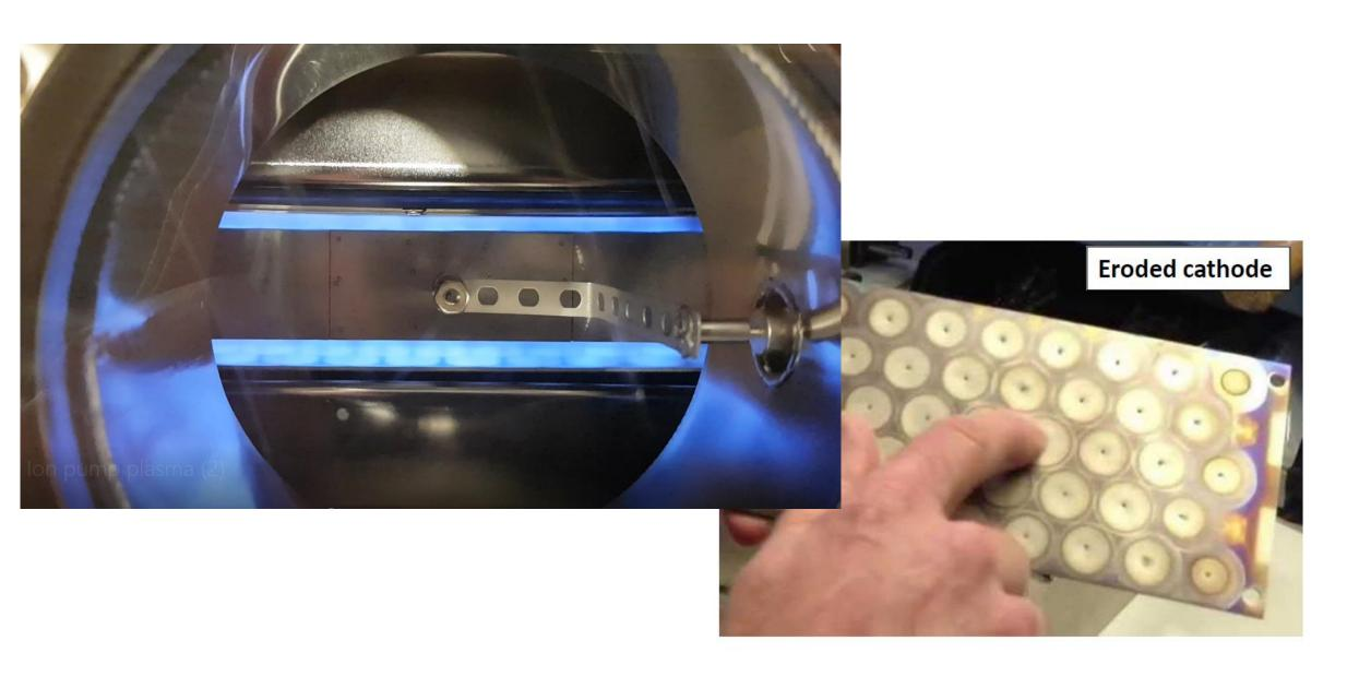
**Lifetime**: cathode is sputtered away (eroded) by impacting ions. If operating at high pressures (10<sup>-4</sup> mbar) the pump lifetime is 400 h whereas at 10<sup>-6</sup> it is 40000 h (4.5 year).
