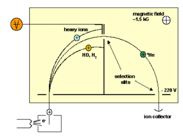
■ Method: helium leak detector
