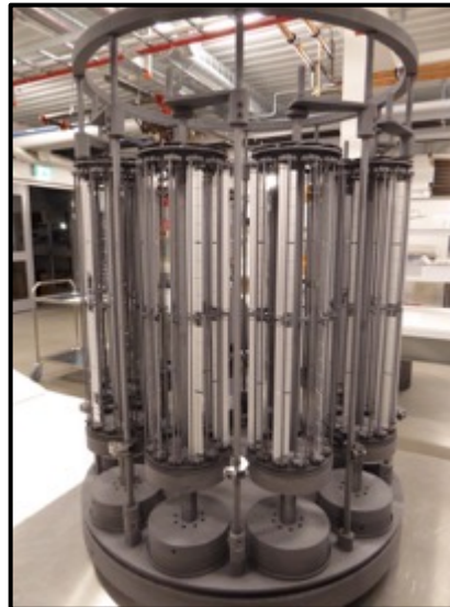
Batch production of B 4 C coated samples
