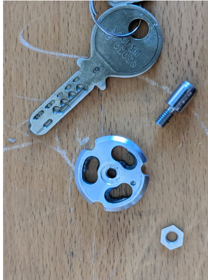
Source: Cs137 - 1.85 GBq Interface Second safety nut
