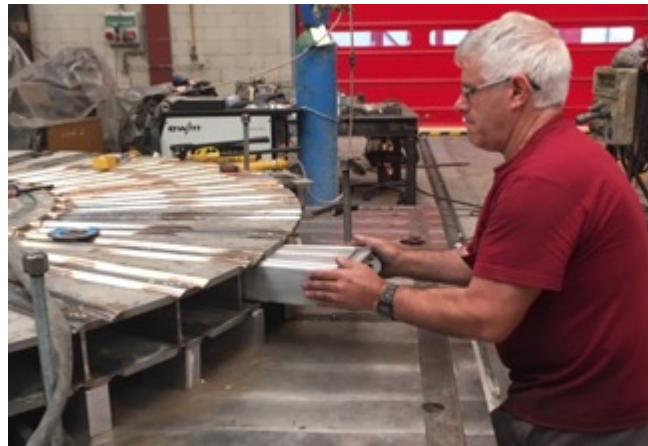
Target wheel ribs in place and finished welding.
