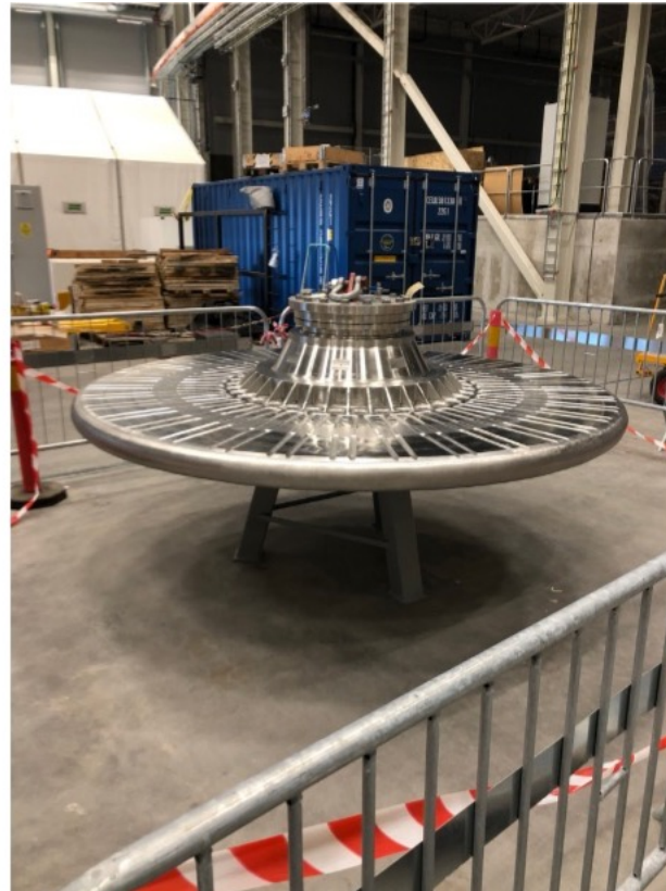
Target wheel assembled in ESS (image does not show shaft)
